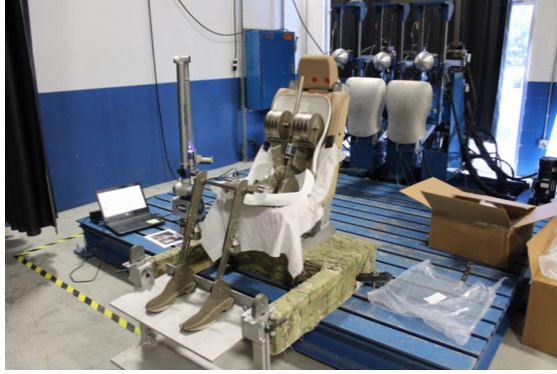
Figure 10. MGA test setup for completing comparative H-point measurements.
