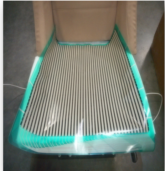
Figure 3. Tekscan pressure mapping sensor placed over seated HybridSil seat cushion within COTS seat pan.
